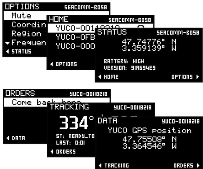
SEACOMM is the communication device with YUCO micro-AUV during mission. Communicating by UHF radio, it allows to received and send message from and to YUCO micro-AUV as soon as its mast is out of water. It can give simple pre-register order to YUCO such as "come back here" and displays micro-AUV last know GPS position.
