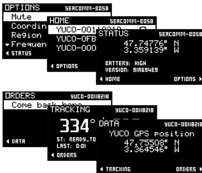
SEACOMM is the communication device with YUCO micro-AUV during mission. Communicating by UHF radio, it allows to received and send message from and to YUCO micro-AUV as soon as its mast is out of water. It can give simple pre-register order to YUCO such as "come back here" and displays micro-AUV last know GPS position.
