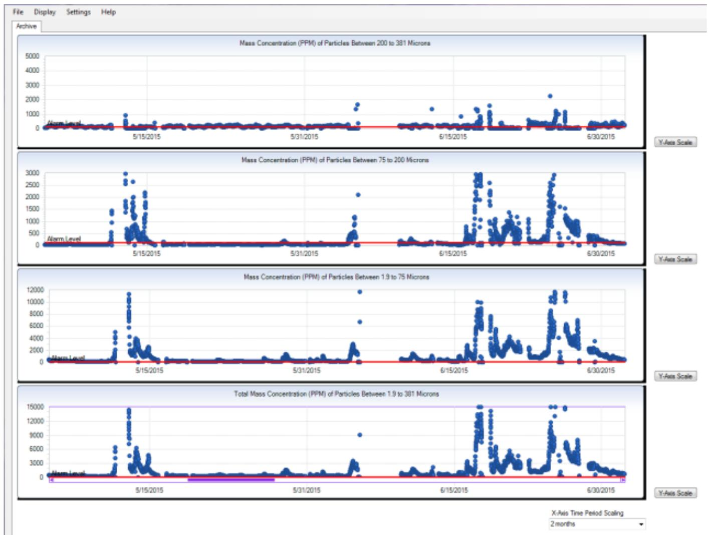
This figure shows a display on plant operator's computer. The strip charts show (from bottom to top) total, fines, medium and coarse grain concentrations. The data are from an actual power plant.
